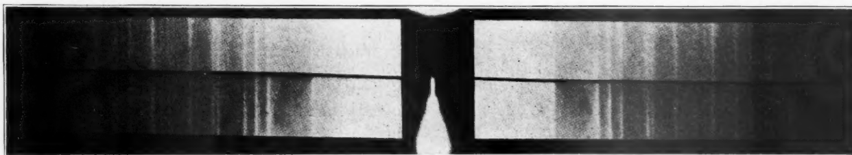
Figure 4—Ca(OH) 2 from Marble Burned in Vacuum; Top, 1800 Degrees Fahr. Bottom, 2400 Degrees Fahr.
